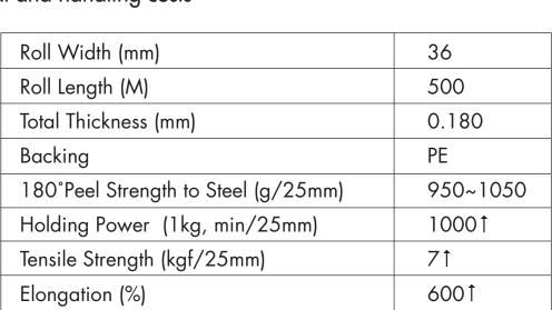
This product should be applied to a clean and dry surface. The above figures represent average values. The selection of a tape is the responsibility of the buyer. Tape should be stored at room temperature and should not be exposed to sunlight. We reserve the right to make changes without notice to our product and specifications.
